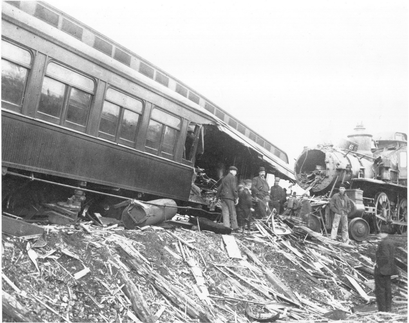
Northbound locomotive No. 69 tangled with a wooden coach after the southbound train split a switch and jumping the track. Photo from the Edward H. Miller Collection
